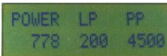
Shows the power consumed by the motor, the low power set point and the peak power allowed.
