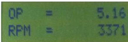
Displays OP which is an internal parameter which may be needed during trouble shooting and also shows the rpm of the motor.
