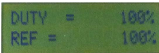
Displays the current duty cycle of the motor, and the maximum duty cycle allowed by the peak power adjustment pot.
