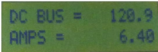
Shows the voltage of the DC input and the current consumed by the pump.
